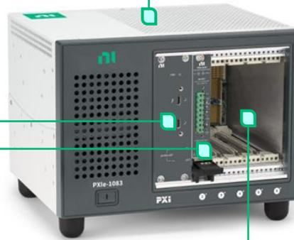
Multi-instrument synchronization by sharing timing and trigger signals through the backplane
